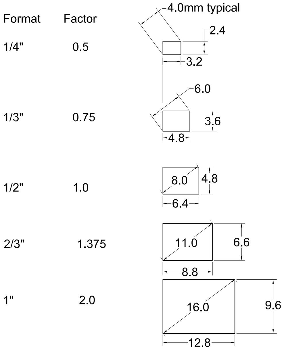
Unless otherwise noted all data is given for 1/2" camera sensors. For FOV or magnification in other sensor sizes use the factors listed. For example, a FOV of 25mm listed for a 1/3" camera would be  $25 \times 0.75 = 18.75\text{mm}$ .
