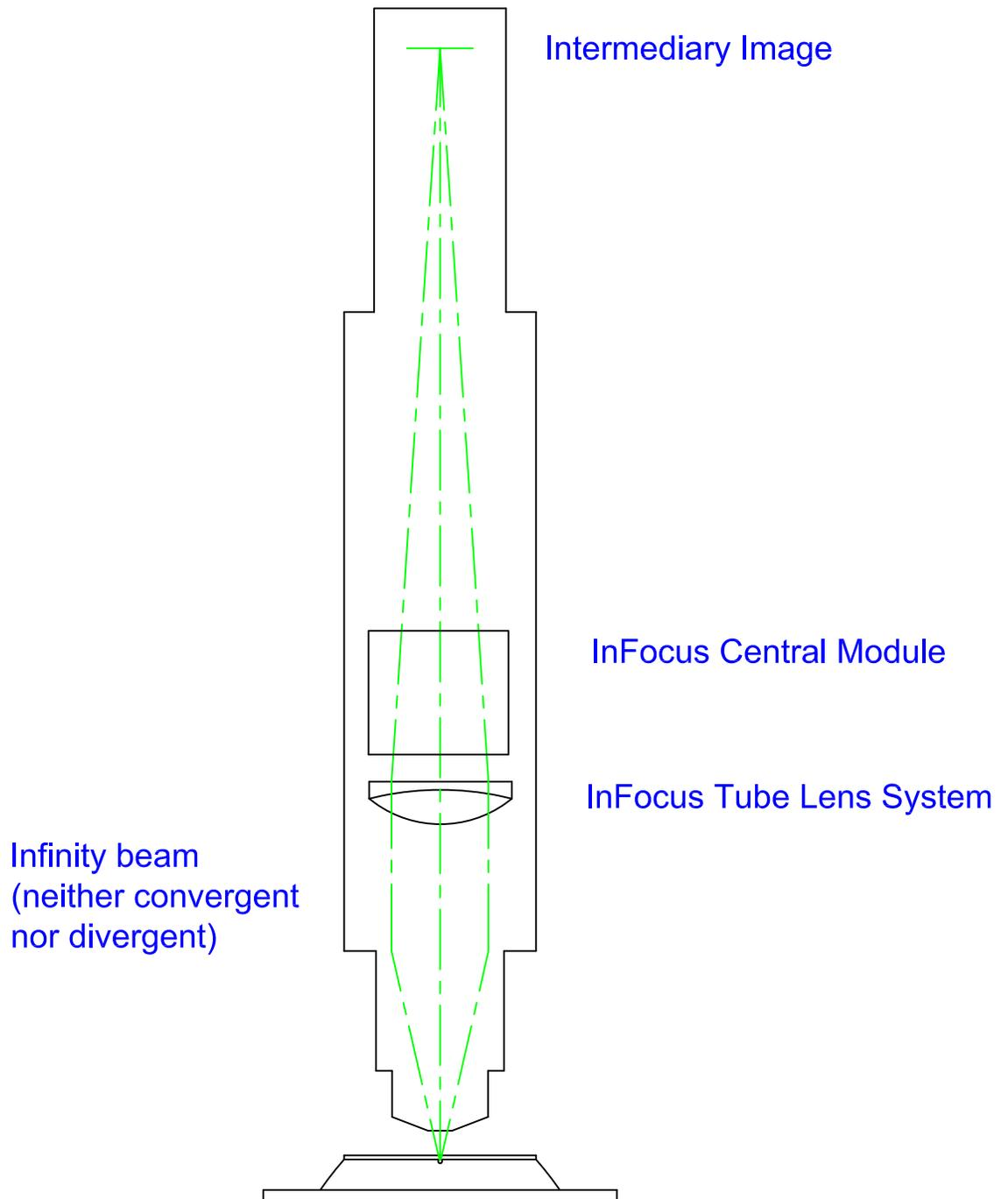
The InFocus module does not work with the Standard Tube Lens.
